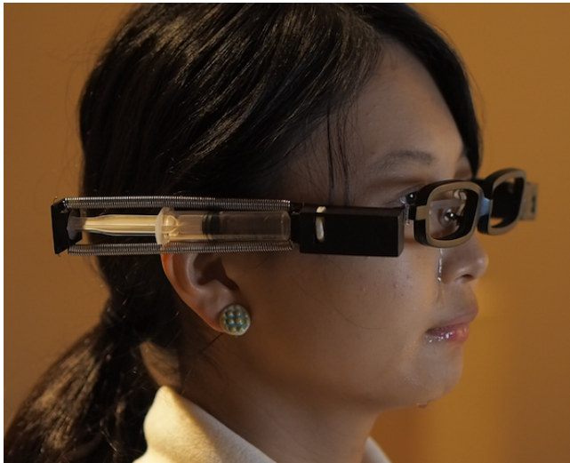
Figure 1: Teardrop glasses: An eyeglasses-style wearable device that aims to trigger emotional contagion with pseudo tears. A drop of water flows onto the face near the inner corners of the wearer’s eyes, and the water flows down his/her cheeks.
